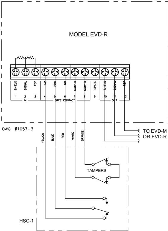
NOTE: The green wire is not used, insulate the loose end.
