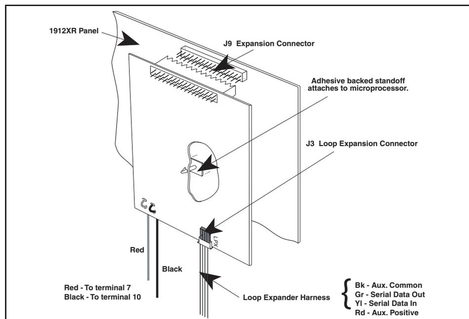
**Figure 1: Installing the 881 on the 1912XR panel**
