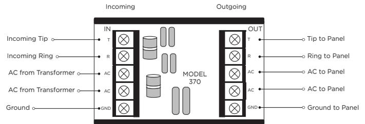
Figure 1: 370 Lightning Suppressor
