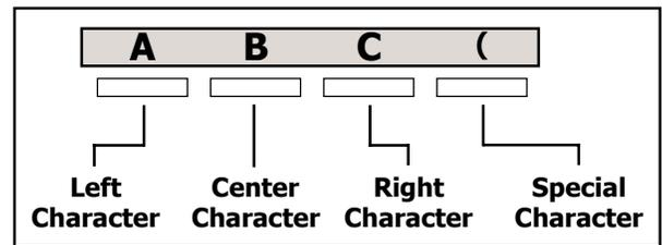
Figure 2: Keypad Display and Select keys
