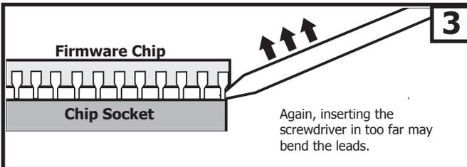
Repeat steps 1 and 2 on the opposite side of the chip. Do not insert the screwdriver too far in between the chip and chip socket when pushing the chip out.
