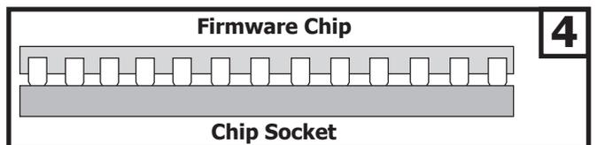
Inspect the PROM to ensure there are no bent leads and the body is level indicating the PROM is fully seated.
