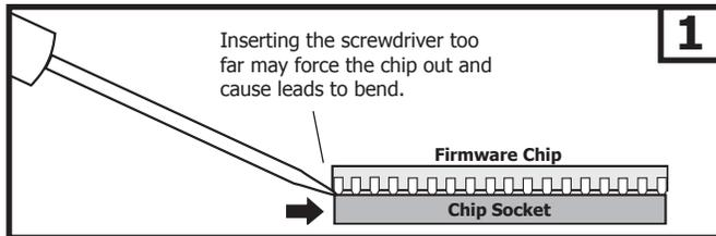
Insert screwdriver between the chip and the chip socket as shown. Start with the side closest to the panel terminals.
