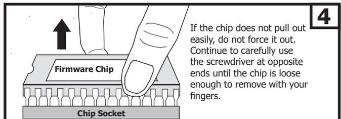
Repeat steps 2 and 3 until the chip is loose enough to easily pull out by hand. Pull with an upward motion to reduce the number of bent leads.
