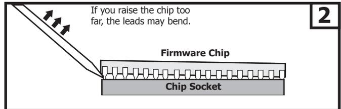
Lift screwdriver while the blade is inserted between the chip and chip socket. Gently push the chip up. Slightly raise the PROM as shown above.
