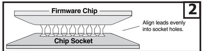
Insert the row of leads farthest from you into the socket holes. Make sure they are aligned.
