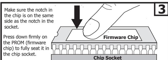
Slowly lower the front row of leads into the socket aligning all leads with the socket holes. Press firmly on the PROM top (firmware chip) until it is fully seated.
