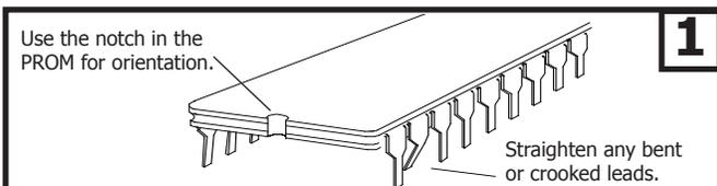
Inspect the PROM (firmware chip) for any bent or crooked leads and straighten gently by hand.
