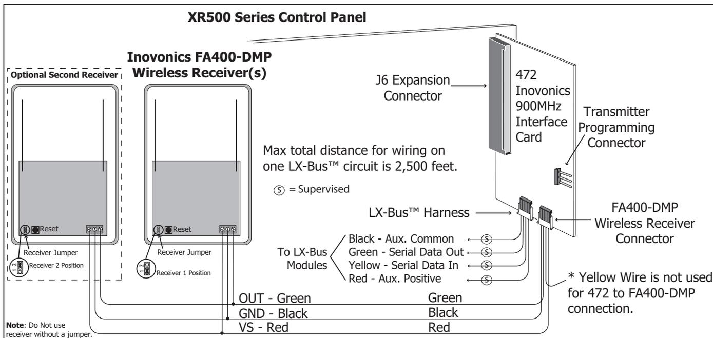
Figure 1: 472 Inovonics 900MHz Interface Card Wiring
