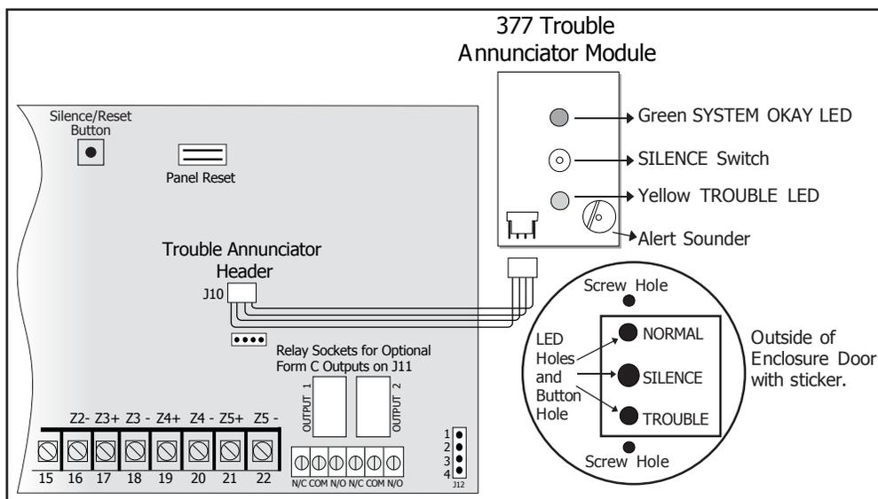
Figure 1: 377 Module Installation and XR5 Fire Panel Connection
