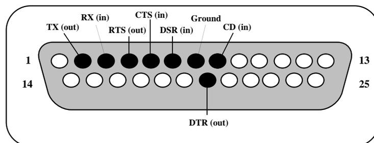
Note: The ETHER-COM DB25 connectors are male. Pinouts for female DB25 connectors are the opposite of this pinout.
