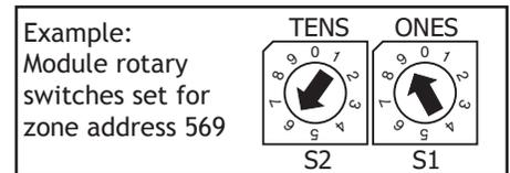
Figure 4: Address switches
