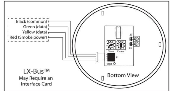
Figure 3: 521LX/LXT Wiring
