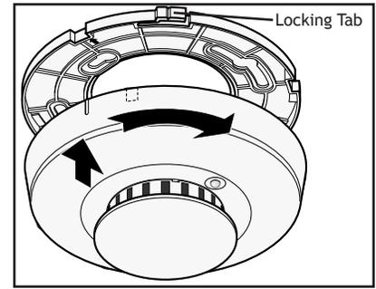
Figure 2: Installing the 521LX/521LXT on the Base
