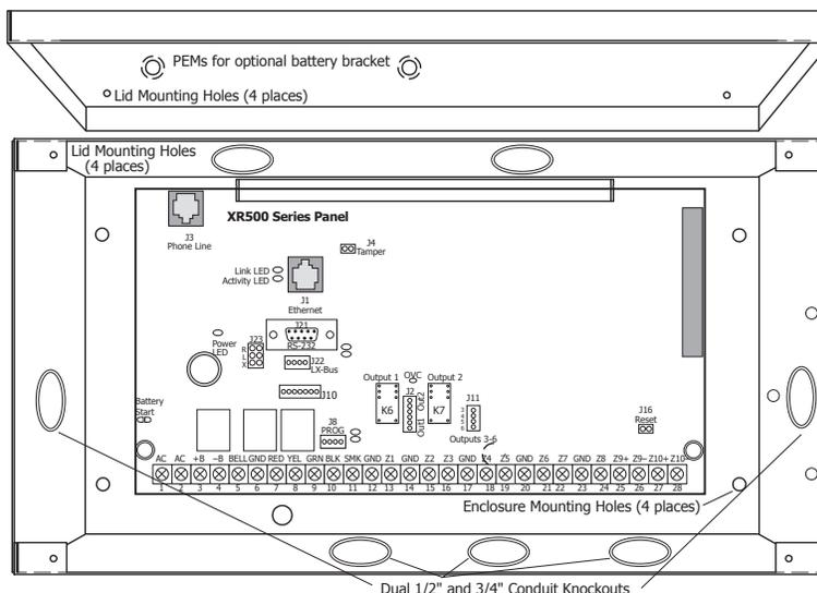
Figure 3: XR500 Series in Model 341 Enclosure
