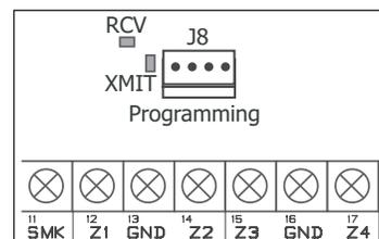
Figure 5: Keypad Bus LEDs
