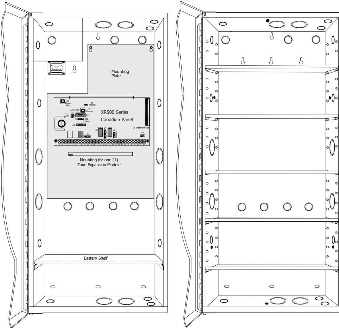
Figure 4: XR500 Series in Model 352X Enclosure and Separate 352S Enclosure with Shelves
