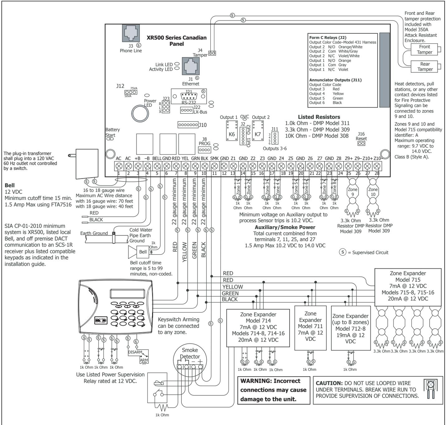
Figure 1: XR500 Series Canadian Wiring Diagram
