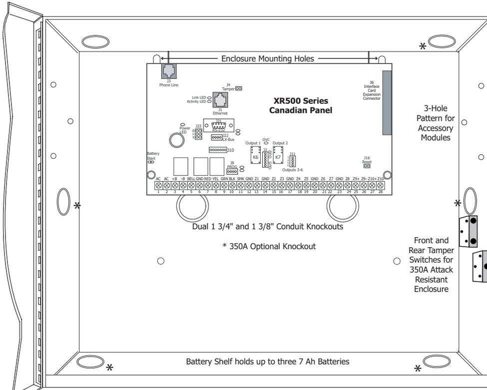
Figure 2: XR500 Series in Model 350 or 350A Enclosure
