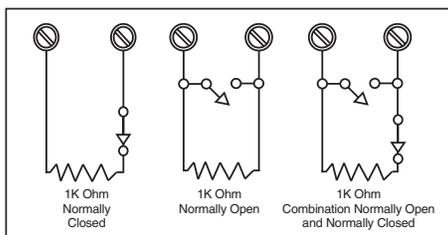
Figure 7: Protection Zone Wiring
