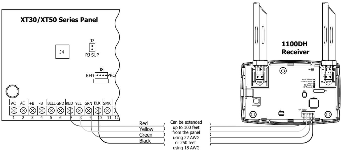
Figure 2: Panel Keypad Bus Connection
