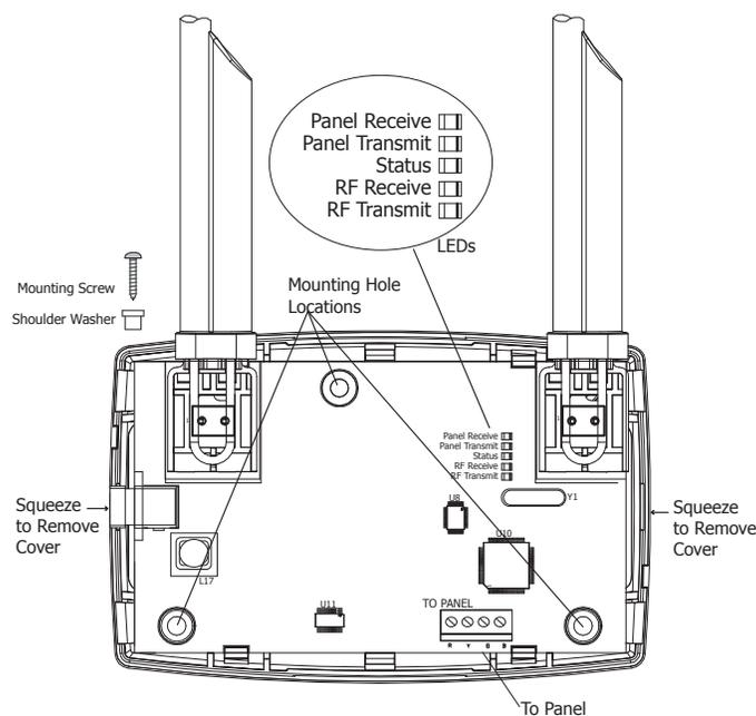
Figure 1: Receiver PCB
