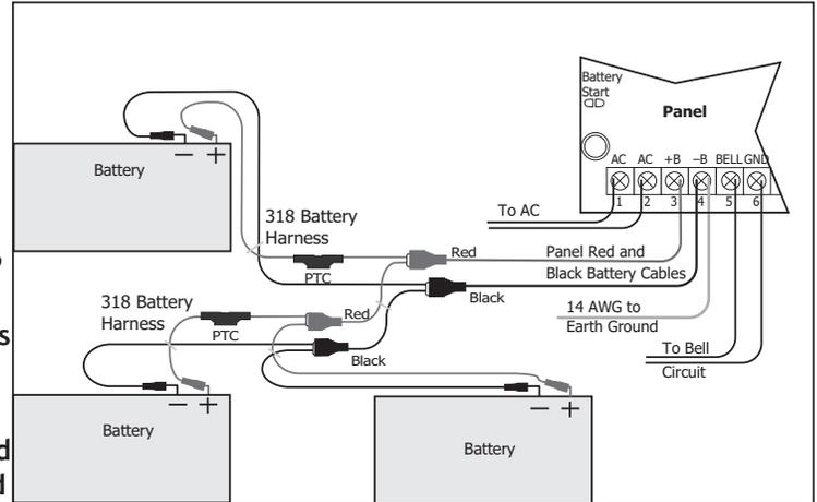
Figure 5: Wiring Multiple Batteries
