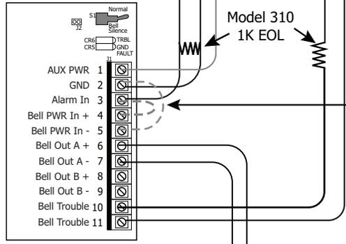
The Bell Output programming for Fire type zones must be set to Temporal.
