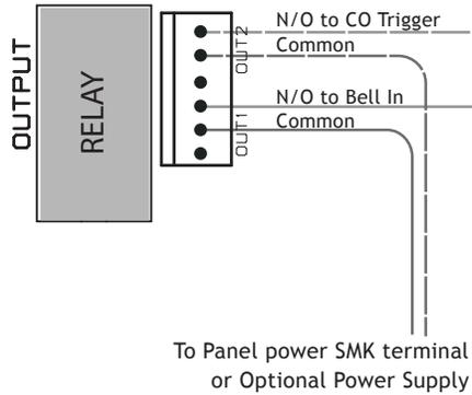
If installing multiple COSMOD2W Interface modules, connect the Bell In terminal to a N/O relay output to turn on ALL COSMOD2W smoke detector sounders during a fire alarm. Connect the Output Common to the panel SMK or optional Power Supply positive terminal (+). In Bell Options, program Bell Output for the relay output number. Program the Bell Output Bell Action as Temporal (T).
