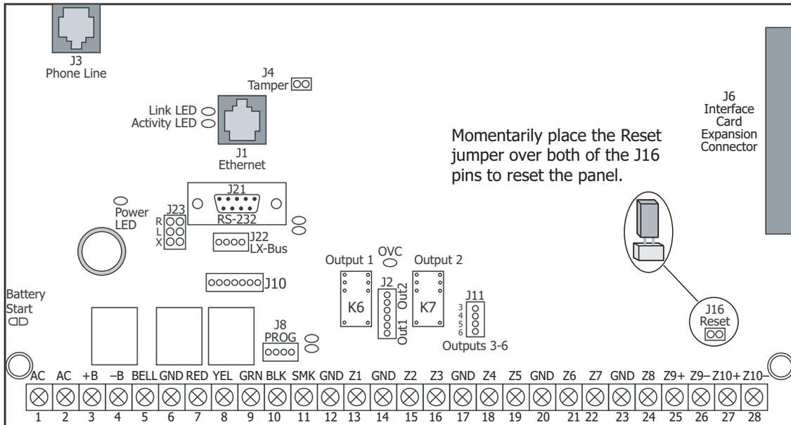
Figure 11: XR500FC Series Panel Showing the Reset Jumper
