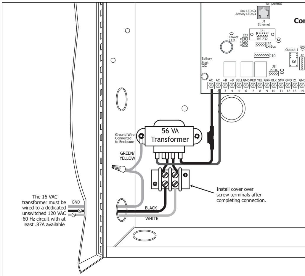
Figure 4: 56 VA Transformer Wiring
