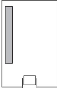
Each LX-Bus Module must have its own independent address ranging from 00 to 99. A Supervisory zone must be programmed into the XR500 Series to properly supervise each module.
