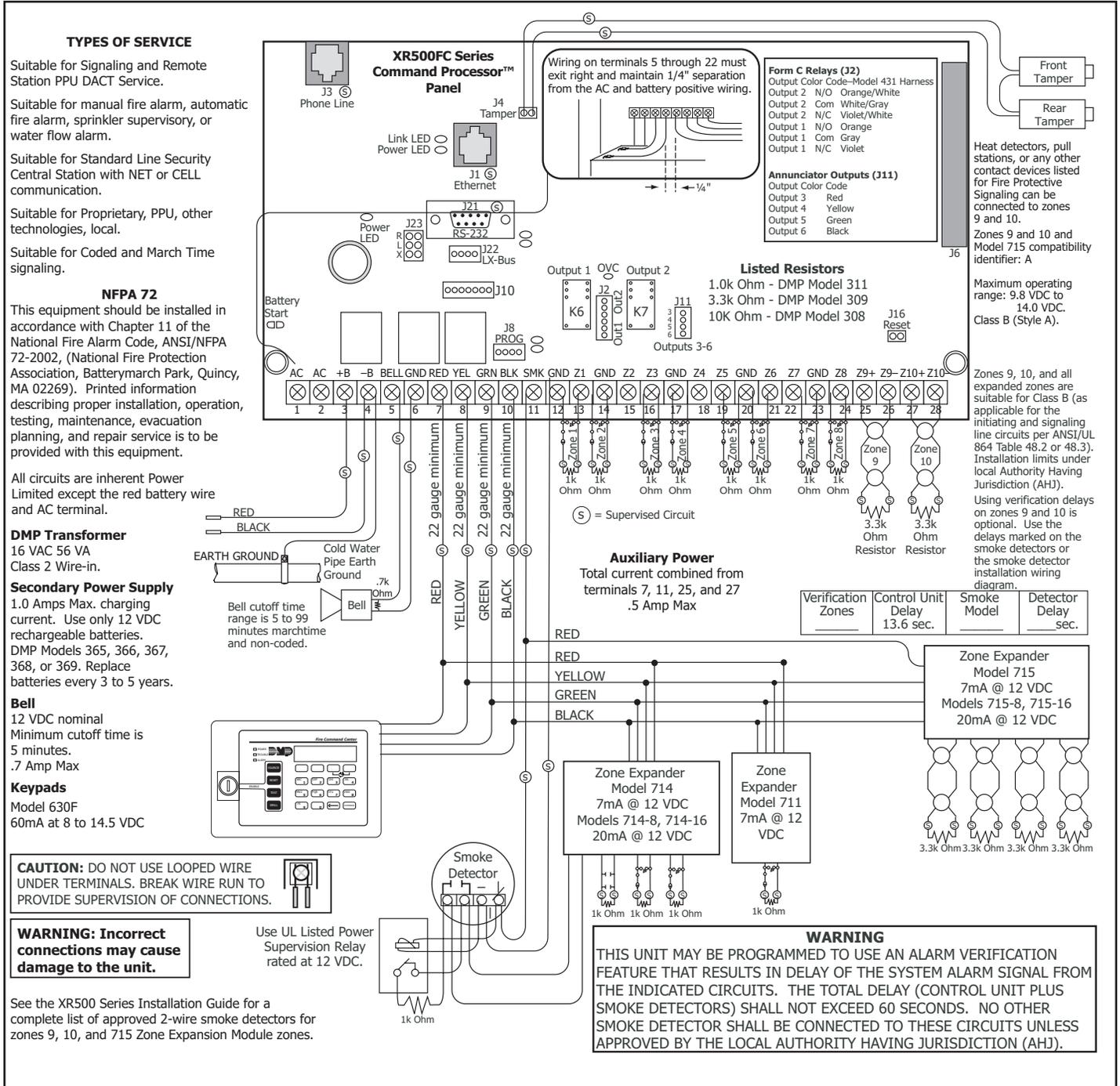
Figure 1: XR500FC Series Wiring Diagram
