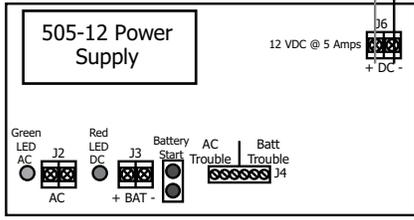
When using a separate power supply, the maximum current is 3 Amps.
