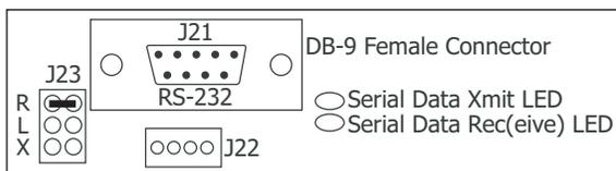
Figure 8: J21 Serial Connection
