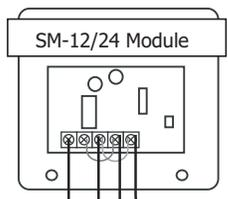
Sync module required when using multiple notification appliances
