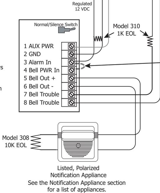
**Note:** Terminals 3 and 4 jumper together to supply Bell Power from the panel
