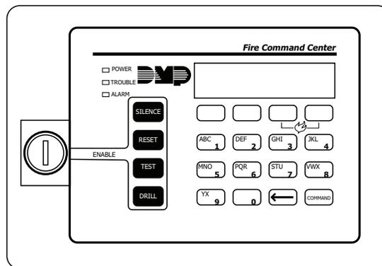
Figure 3: Fire Command Center LCD and Keyboard
