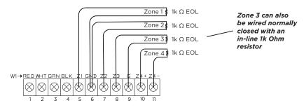
Figure 9: Zone Terminal Wiring
