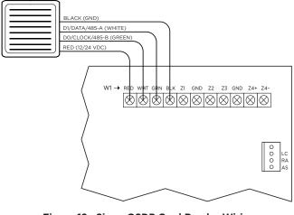
Figure 12: Signo OSDP Card Reader Wiring
