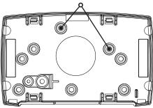
Figure 2: Mounting Hole Locations
