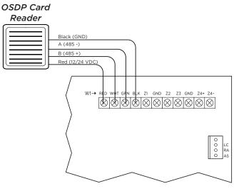
Figure 11: OSDP Card Reader Wiring
