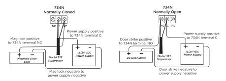
Figure 3: Typical Magnetic Lock Wiring
