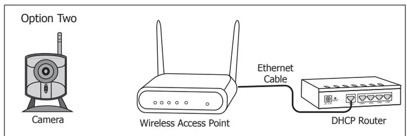
2. Press the WPS button on the front of the WAP for 3 seconds. The Security LED will flash to indicate that the WAP is sending a security key to the wireless camera.
