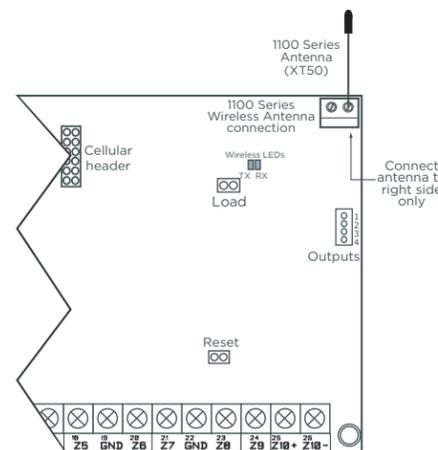
Figure 1: Wireless Antenna
