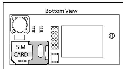
Figure 1: 263H SIM Card Installation
