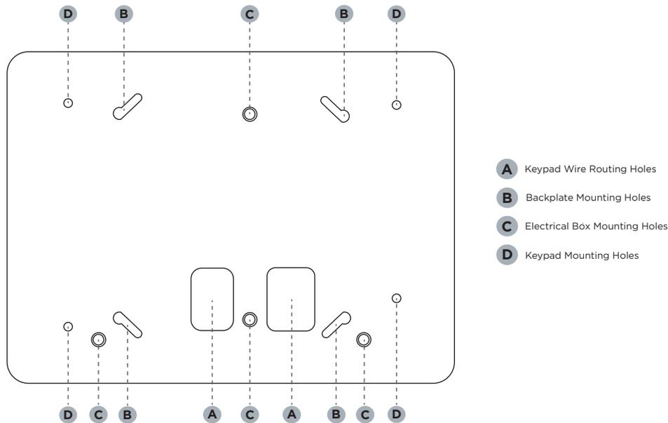
Figure 1: Mounting Hole Locations
