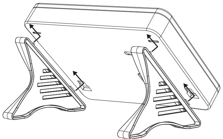
Figure 3: Deskstand Installation
