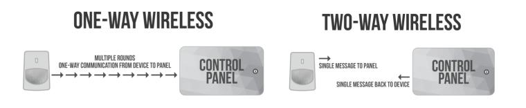
DMP two-way communication enables the control panel and sensors to exchange information. This allows the wireless devices to be controlled and adjusted remotely from the panel or Remote Link<sup>™</sup> software. DMP Two-Way technology sends a single message and immediately receives a single acknowledgement signal allowing it to save much needed battery life.
