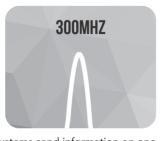
300MHz systems send information on one narrow band channel which results in a more cluttered band causing missed signals.
