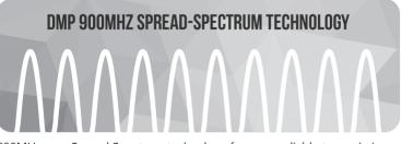
900MHz uses Spread Spectrum technology for more reliable transmission which allows numerous channels within the 905-924 MHz band to be used to ensure a reliable signal.
