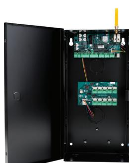
Each X1-ELEV controls access to 10 floors. A single X1 can support up to nine of these modules, meaning you can give your customers up to 90 floors of access control.
