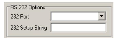
**232 Setup String:** This option displays when the Communication Type is RS-232. Enter up to a 32 character modem string.
