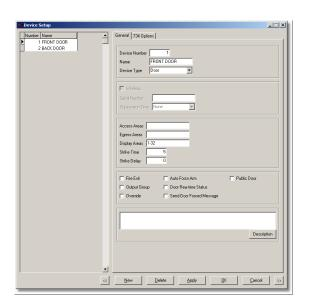
**Device Type:** Specify the type of device installed at a particular address on the keypad bus.
