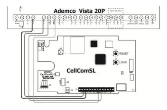
ECP operation must be enabled in the CellComSL. See Keypad Input and the Ademco/Honeywell panel wiring diagram example in the CellComSL Installation/Programming Guide (LT-1339) for additional information.
