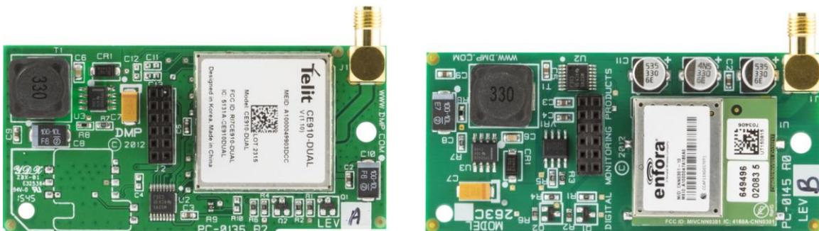
Additional Information: The Model 464-263C Cellular Communication Module will continue to be manufactured using the Enfora modem to remain compatible with the older XR100 and XR500 Control Panels.
