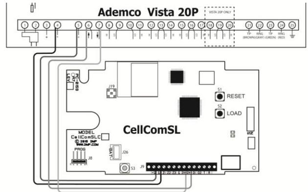
ECP operation must be enabled in the CellComSL. See Keypad Input and the Ademco/Honeywell panel wiring diagram example in the CellComSL Installation/Programming Guide (LT-1339) for additional information.
