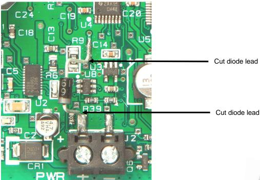
Discard the diode, reassemble and test the XTLC.
