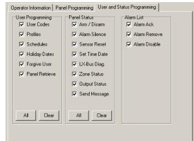
**Alarm List**: Check the box for each operator to have authority to acknowledge, remove, or disable alarms. When upgrading from previous Remote Link versions the alarm authority options are automatically enabled.
