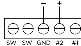
Figure 2: Pulse Tone Wiring
