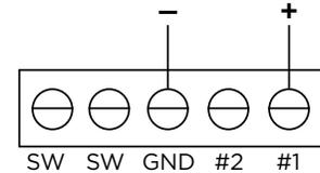
Figure 3: Steady Tone Wiring
