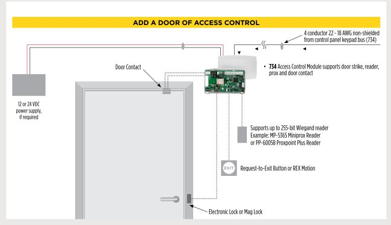
Unlike the access control capabilities of our XR Series™ panels, the door access capabilities of the XT panel are basic. The biggest advantage of XT50 door access is the ability to easily grant access to doors electronically. Concerns of unreturned keys and key duplication are eliminated by using this functionality. On the XT50 panel, all enrolled cards will work on all system readers at all times.
