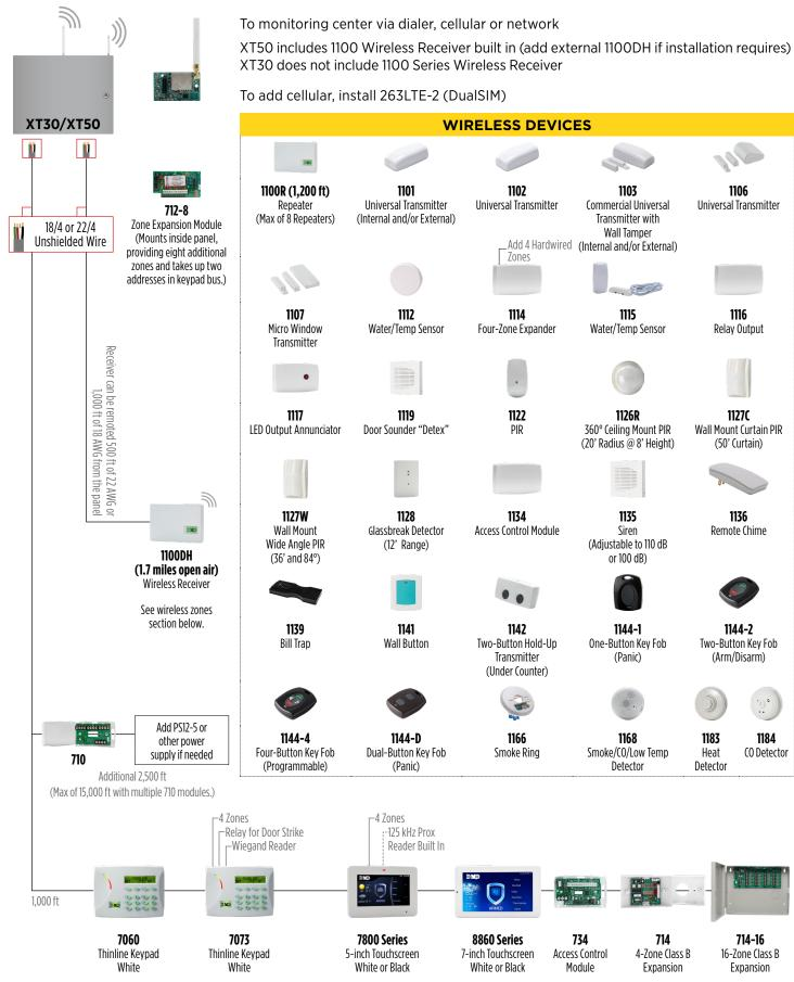
Zone expanders use up one address for every four zones. Example: A 714-8 takes up two of the available keypad bus addresses.
