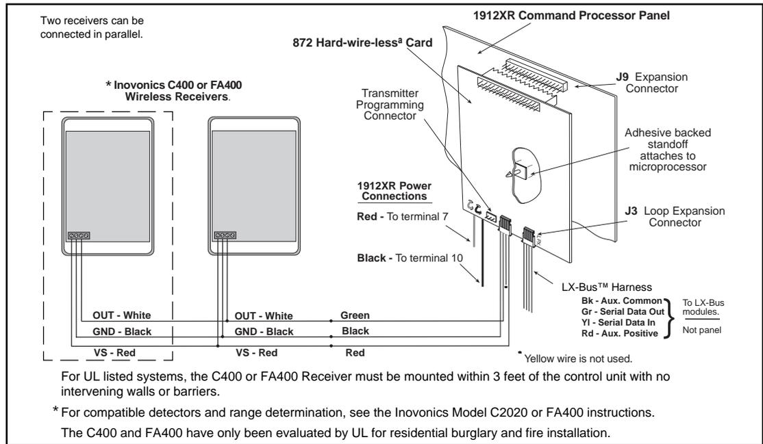
**Figure 1: Wiring for the 400 series receiver(s) and 872 card.**
