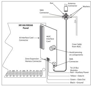
Figure 1: Install and connect the 463C and Antenna
