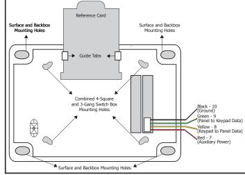
Figure 1: 692F Wiring and Mounting Diagram
