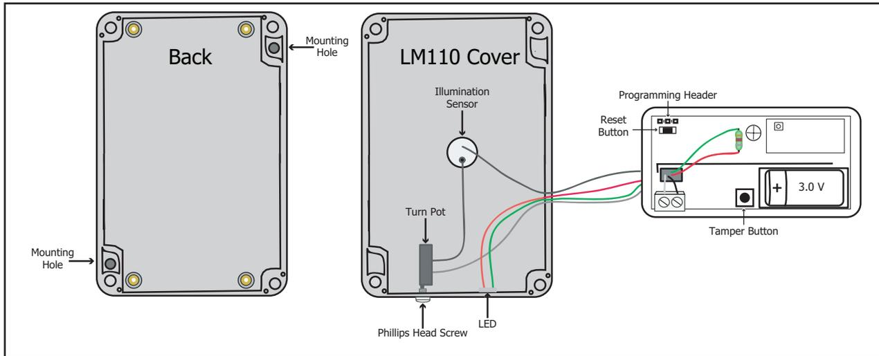
Figure 1: LM110 Wiring Diagram
