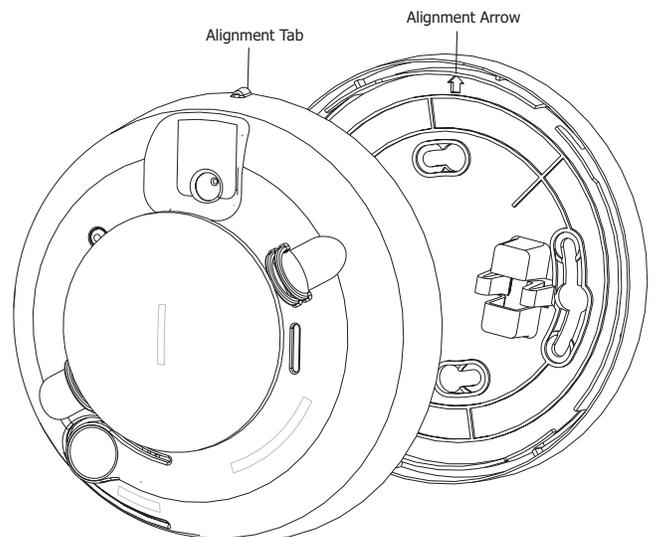
Figure 4: Smoke Detector-to-Base Alignment
