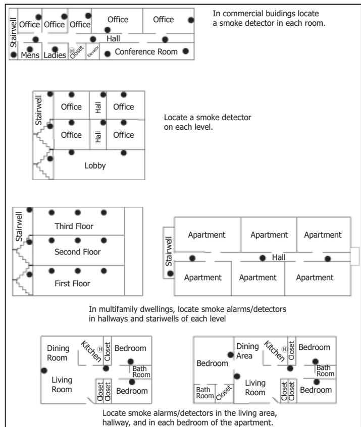
Figure 2: Smoke Detector Placement Locations
