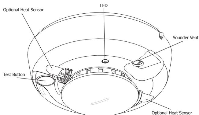
**Figure 1: Smoke Detector Features**
