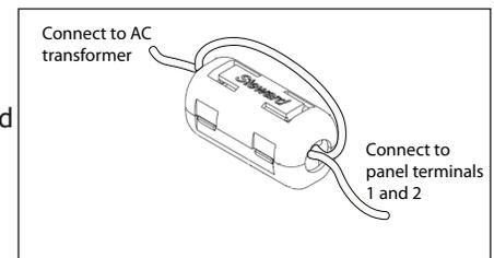
Figure 2: Ferrite Core
