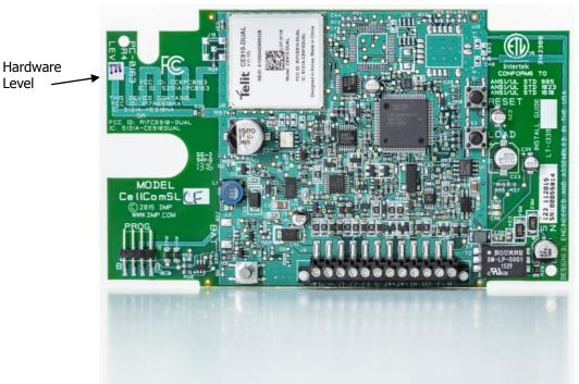
CellComSLCF PCB hardware prior to Level E cannot be updated to this new level. CellComSLC and CellComSLCZ communicators will transition to Level E hardware when current inventory is depleted which is estimated to occur in September 2016.
