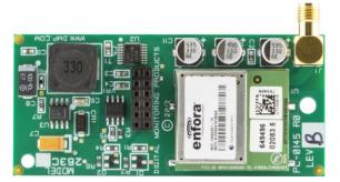
Additional Information: The Model 464-263C Cellular Communication Module will continue to be manufactured using the Enfora modem to remain compatible with the older XR100 and XR500 Control Panels.
