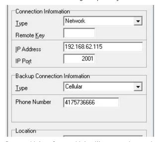
Remote Link or System Link will try two times using the primary information before attempting to connect to the panel using the Backup Connection Information. "Switching to backup connection." displays bold and red when the primary connection has failed. Remote Link or System Link will try two times using the backup information before aborting connection.
