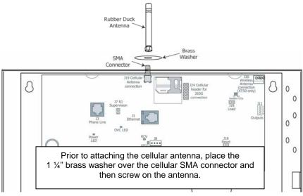
If additional washers are needed for any existing installations they are available from DMP free of charge. Please contact DMP customer service at 1-800-641-4282 and request part number FP-0142.
