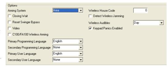
during sleeping hours (9 PM to 9 AM). Select MIN (minimum) to annunciate only Fire and Fire Verify zones during daytime hours (9 AM to 9 PM). Default is DAY.
