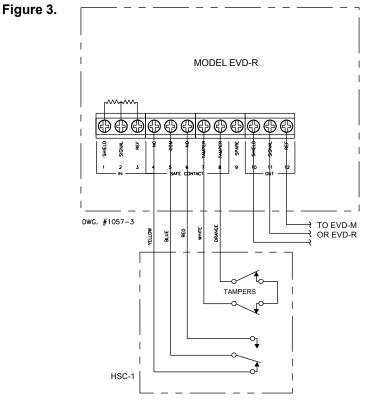
NOTE: The green wire is not used, insulate the loose end.
