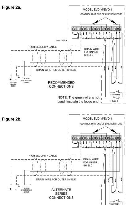
NOTE: The green wire is not used, insulate the loose end.
