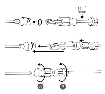
Figure 2: Installing the Waterproof Ethernet Cap
