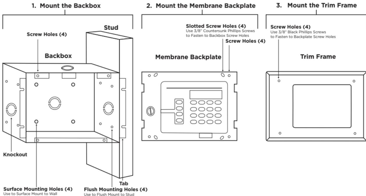
**Figure 2: Mounting Diagram**
