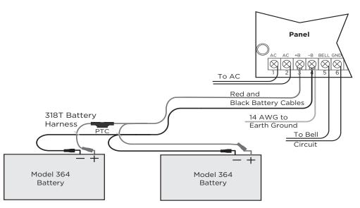
**Figure 4: Wiring Multiple Batteries**
