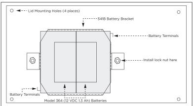
Figure 3: Model 341 Enclosure Lid and Model 341B Battery Bracket
