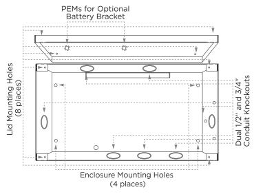
Figure 2: Mounting holes
