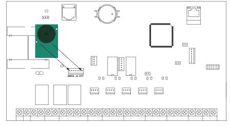
Figure 2: 277CAN Trouble Sounder to Panel Connections
