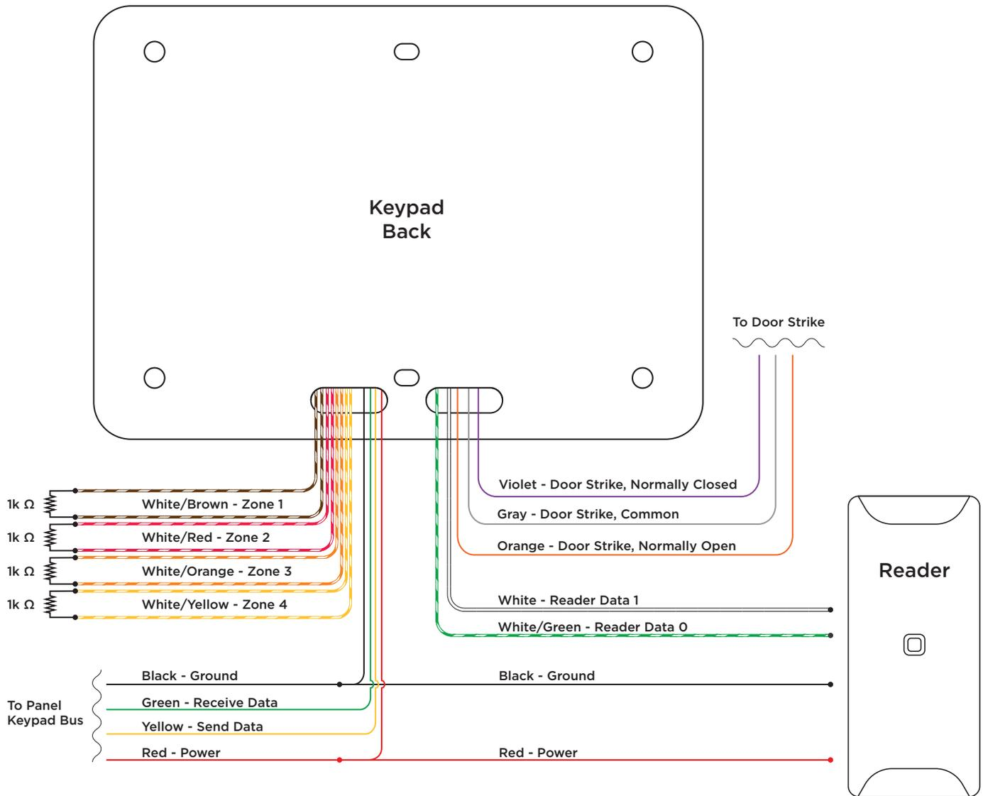
Figure 3: Keypad Wiring
