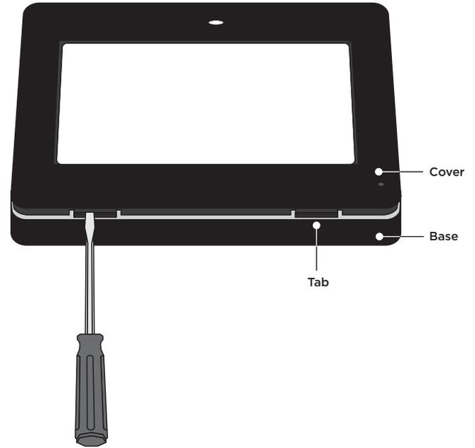
Figure 1: Removing the Cover
