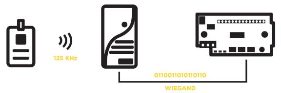
To ensure compatibility with DMP access control, the credential, card reader and door controller are the three primary components to consider. In this illustration, a 26-bit credential uses the 125-kHz frequency to transmit its data to the card reader, which relies on the Wiegand output module to communicate with the door controller.
