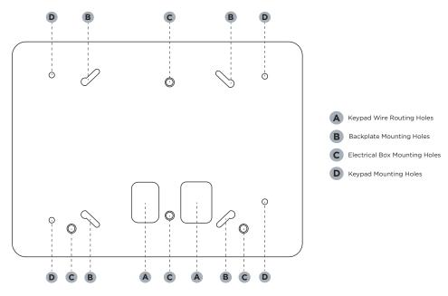
**Figure 1: Mounting Hole Locations**
