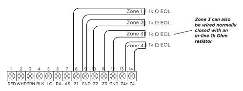
Figure 8: 734B Zone Terminal Wiring
