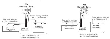
Figure 3: Typical Magnetic Lock Wiring
