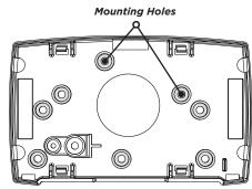
Figure 2: Mounting Hole Locations
