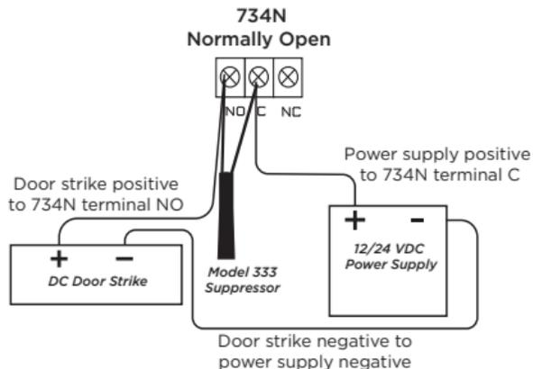
**Figure 4: Typical Door Strike Wiring**
