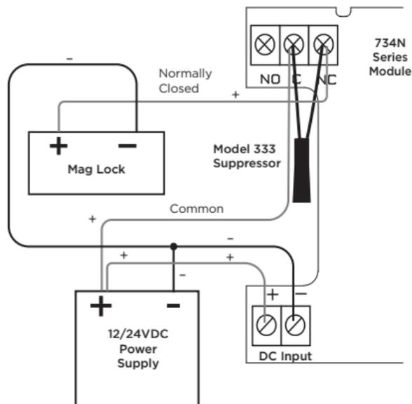
**Figure 6: Magnetic Lock with an Isolation Relay**
