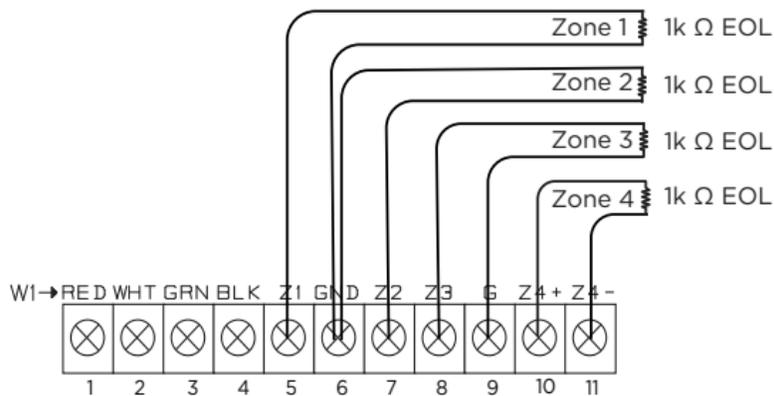
*Zone 3 can also be wired normally closed with an in-line 1k Ohm resistor*
