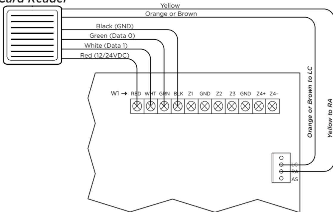
**Figure 10: Wiegand Card Reader Wiring**
