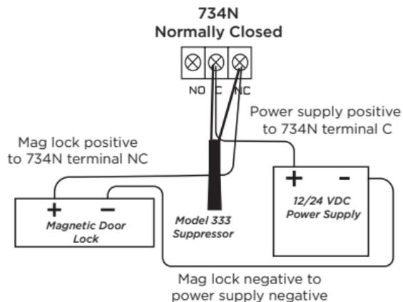
**Figure 3: Typical Magnetic Lock Wiring**
