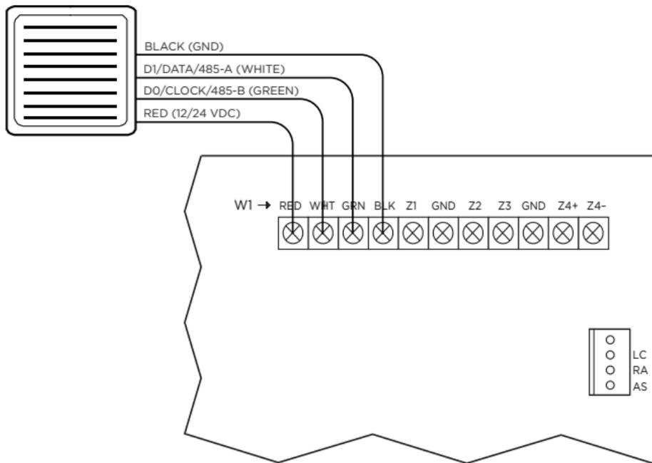
**Figure 12: Signo OSDP Card Reader Wiring**
