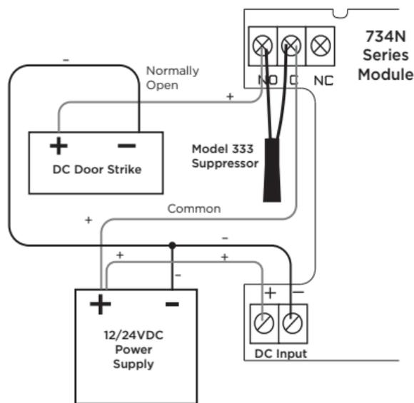
**Figure 7: Door Strike with an Isolation Relay**
