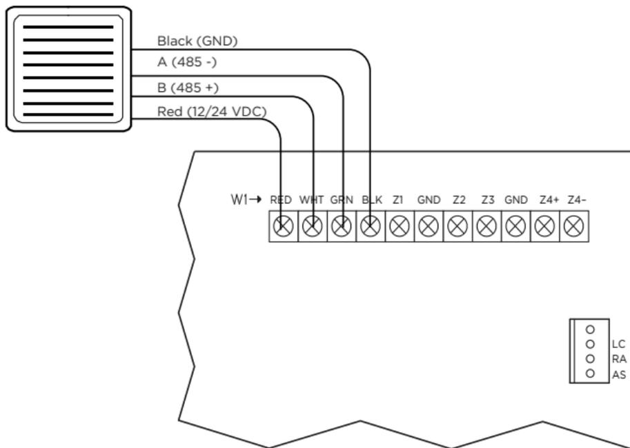
**Figure 11: OSDP Card Reader Wiring**
